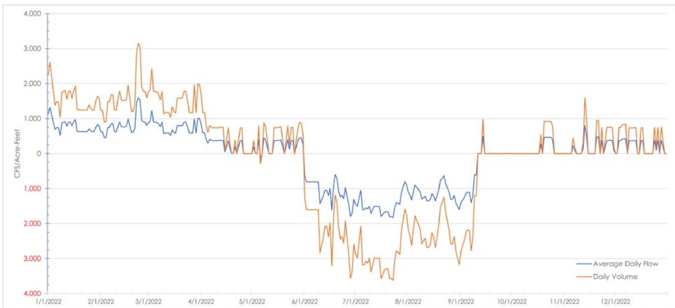
Lake Pleasant average daily inflow/outflow (cfs) and volume (acre-feet). Positive levels represent when water is pumped into Lake Pleasant from the CAP (pumping), while negative values represent when water is discharged from Lake Pleasant into the CAP canal (generating).
