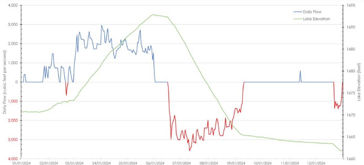
Lake Pleasant average daily inflow/outflow (cfs) and lake elevation (feet). Positive levels represent when water is pumped into Lake Pleasant from the CAP (pumping), while negative values represent when water is discharged from Lake Pleasant into the CAP canal (generating).
