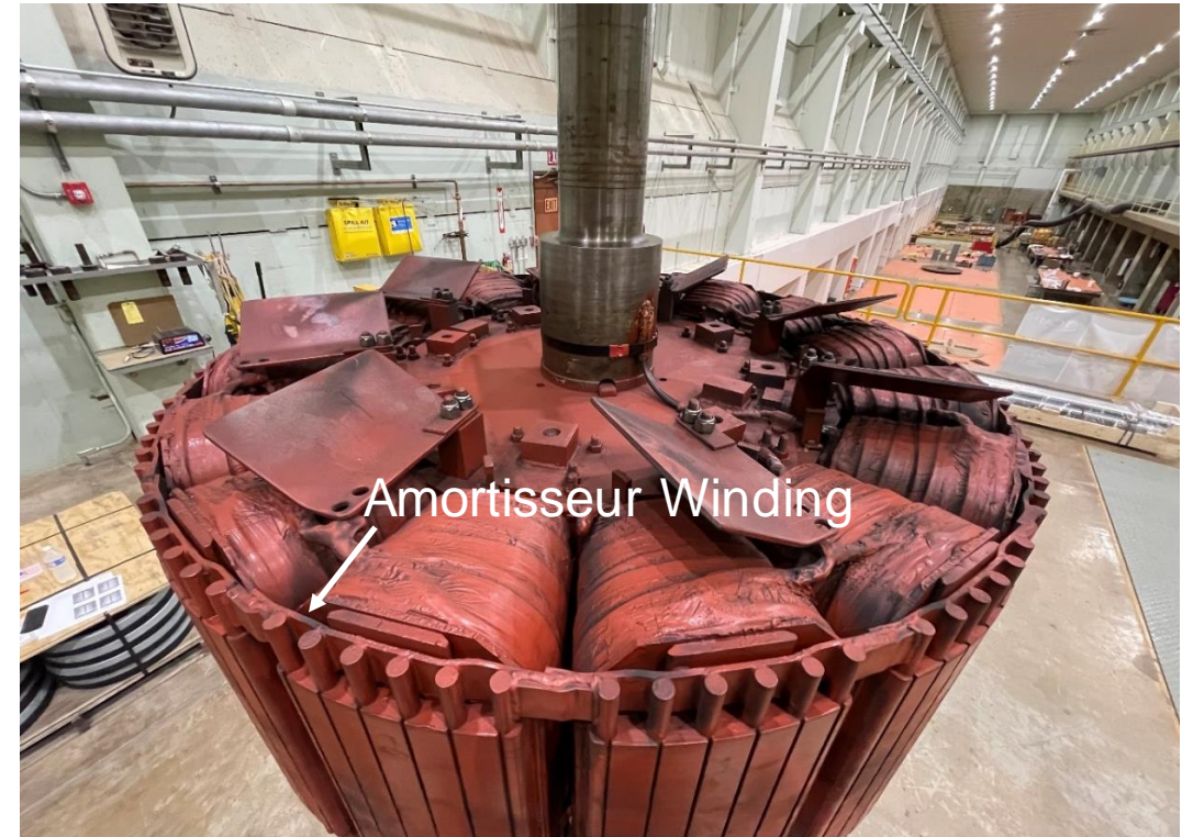
LHQ U10 Rotor 2250 HP Electric Motor
