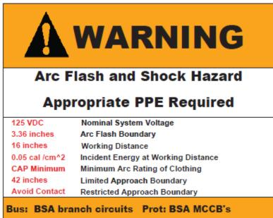
Example of an electrical hazard label on equipment that has not had an incident energy analysis performed. Arc flash boundary and PPE requirements determined from NFPA 70E Tables 130.7(C)(15)(a) and (b). See <u>Appendix D</u>
