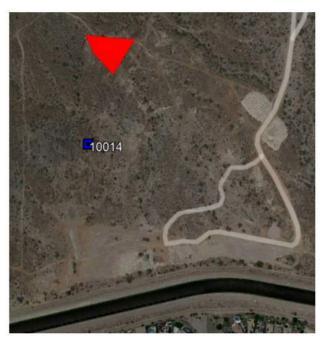
When the blasting is taking place within 500 feet of the canal, monitor(s) must be placed at the perimeter fence for the canal, or at the top of the concrete lining of the canal at the request of CAWCD. If the Canal is in a concave bend and there are two possible close points, there shall be two monitors placed at each of the locations as shown below:
