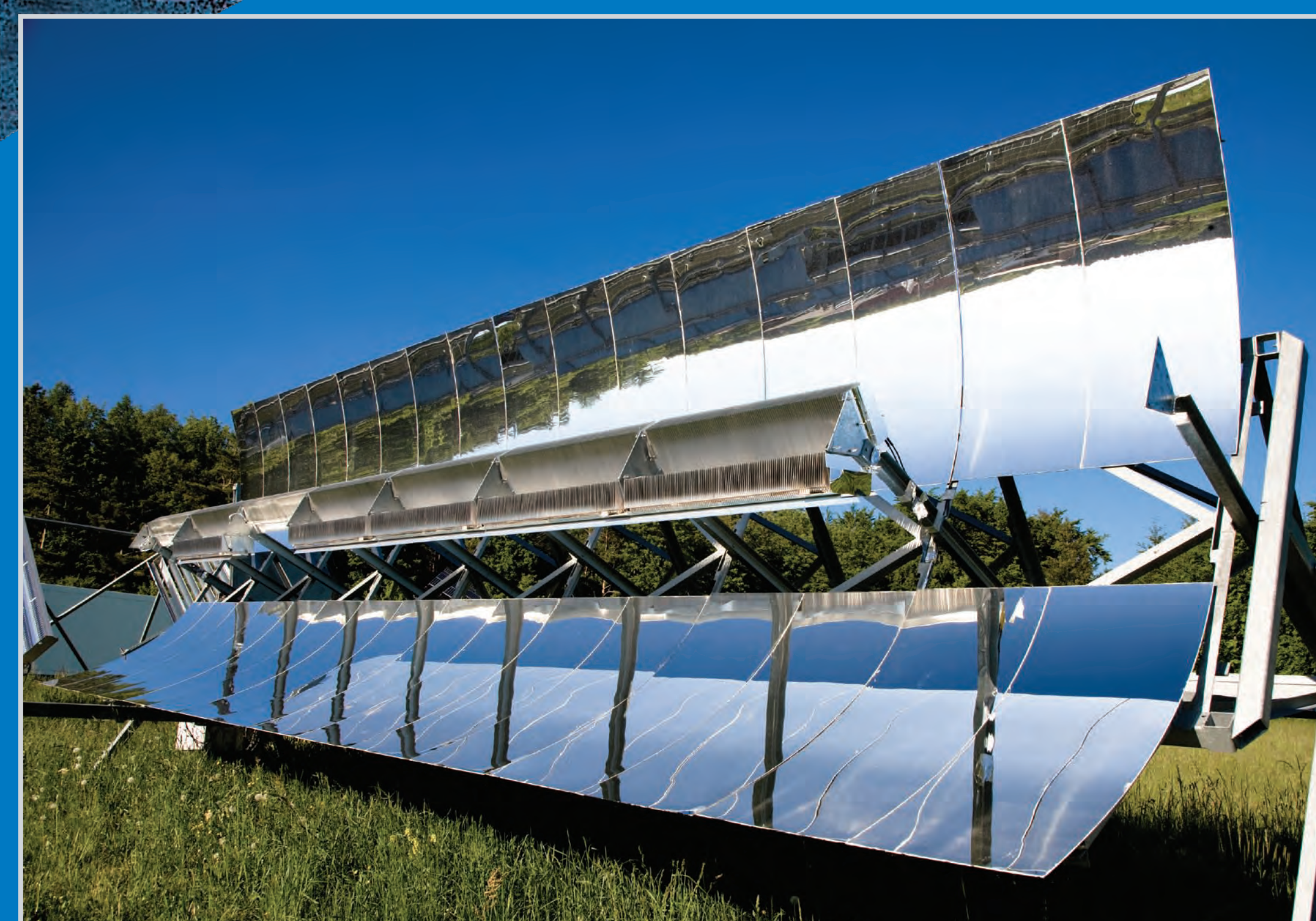
Close-up of a parabolic trough showing collector tube containing oil at trough focal point.
